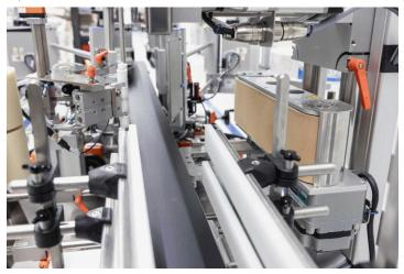
The innovative design of the 362E makes the **changeover from two-sided labeling to wrap-around labeling** easier than ever before.
